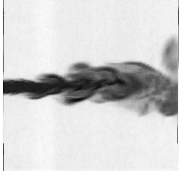
Fig. 2 Instantaneous passive scalar contours produced by dynamic Smagorinsky model on an xy plane, z = 8 .
